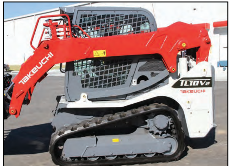
Vertical Lift Path for Balance and Stability
